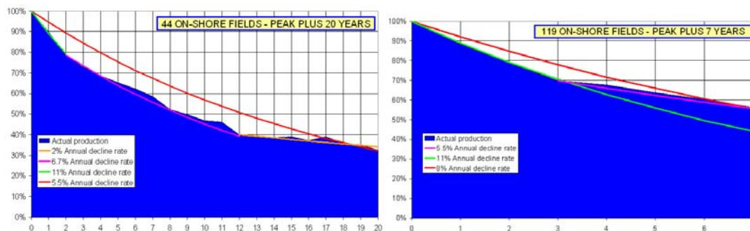
Figure 3.6: Onshore field decline, for 20 years, (left) and 7 years (right) after peak production. The red curve in each chart is a single, fixed, approximate decline curve, but the actual decline rate falls with time
