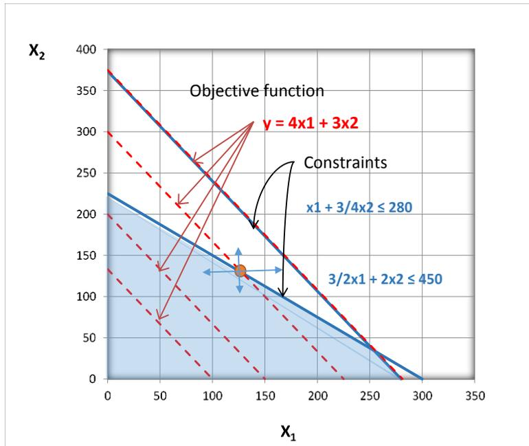
Figure 5. Schematic representation of linear program example
