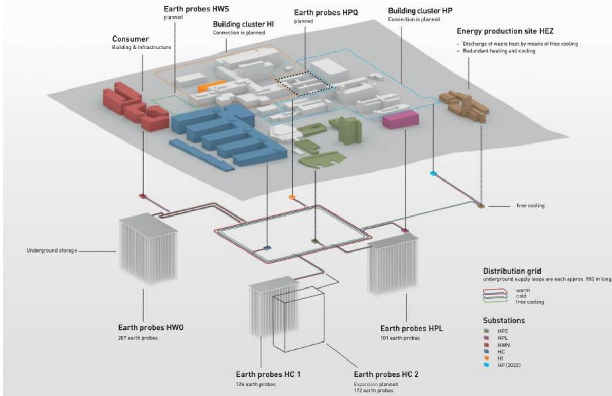
Figure 15. Illustration of the Anergy Grid, from [19]
