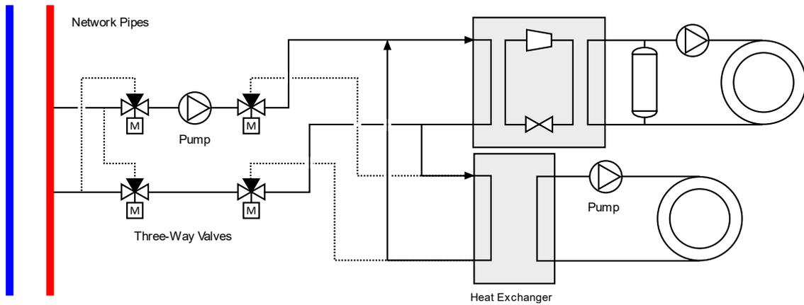
**Figure 11. Basic substation layout for active heating using a dedicated water-source heat pump and indirect passive cooling using a heat exchanger. A buffer tank and bi-directional network exchange via three-way valve arrangement also feature. The layout permits direct interchange of heat between heating and cooling loads. A similar layout would be used for active cooling with passive heating.**
