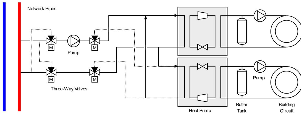
**Figure 10. Basic substation layout for active heating and cooling using dedicated water-source heat pumps, buffer tanks and bi-directional network exchange via three-way valve arrangement. The layout permits direct interchange of heat between heat pumps**
