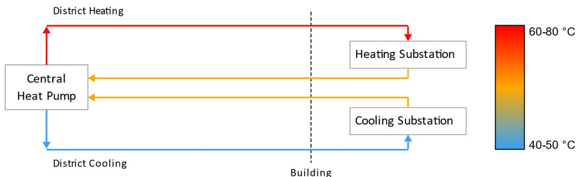
**Figure 6. Illustrative layout for the Warm – CHC configuration, redrawn from [9]**
