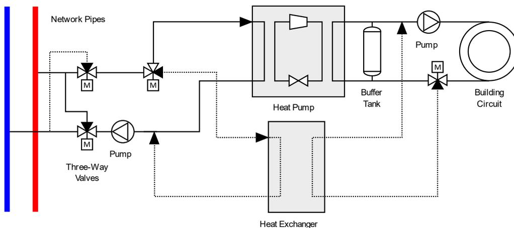
**Figure 13. Basic substation layout for active heating and passive cooling for cases where loads are not coincident. Features a water-source heat pump, heat exchanger, buffer tank and bi-directional network exchange via three-way valve arrangement. A similar layout would be used for active cooling with passive heating**
