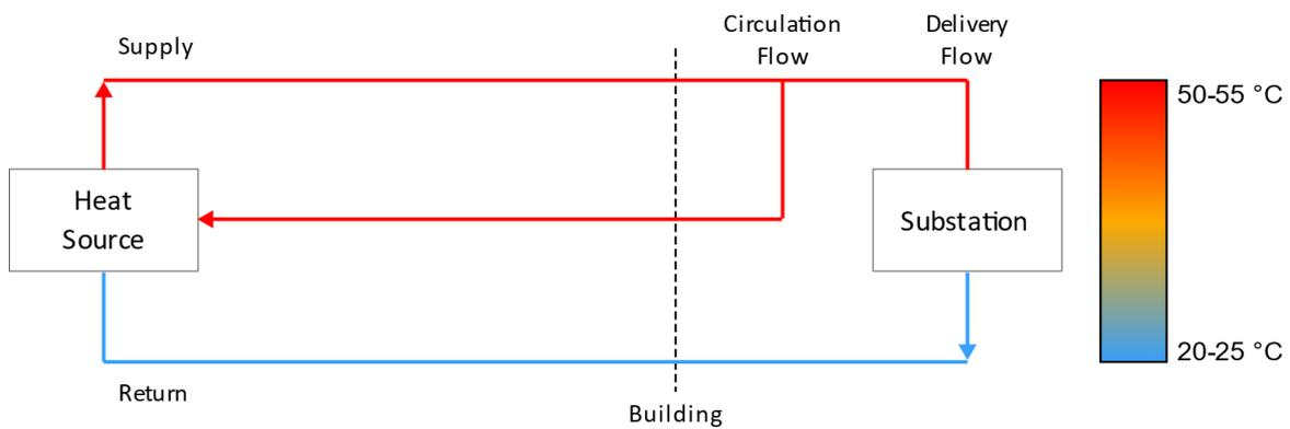
**Figure 3. Illustrative layout for the Warm – Modified Classic configuration, redrawn from [9].**
