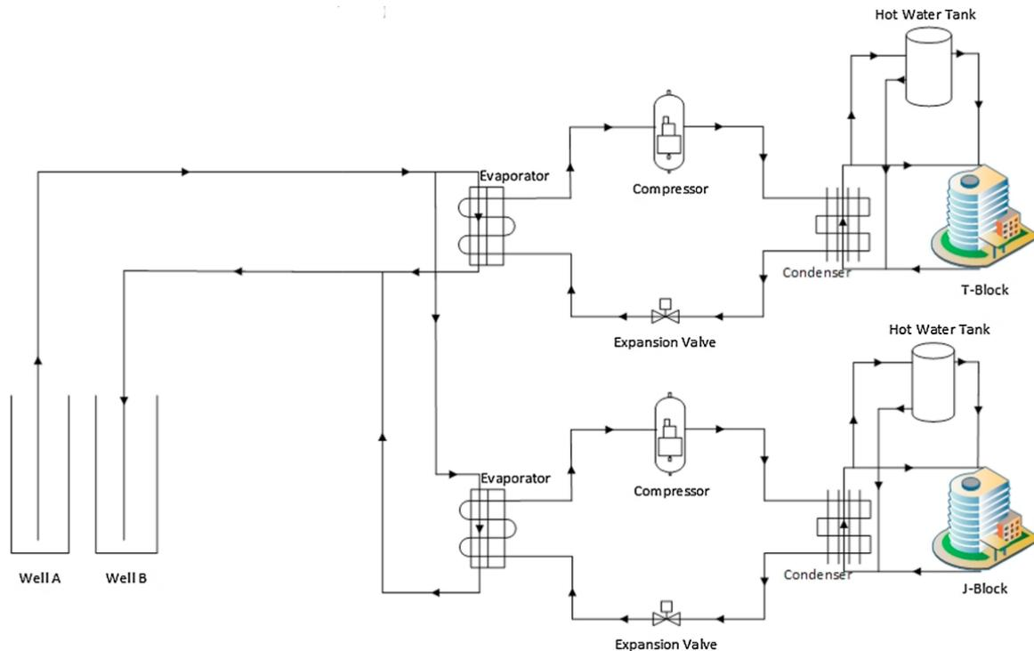
Figure 16. Schematic of the Balanced Energy Network, from [21]
