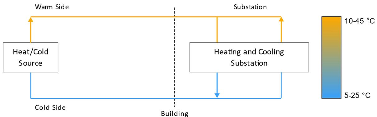
**Figure 9. Illustrative layout for the Cold – CHC configuration, redrawn from [9]**
