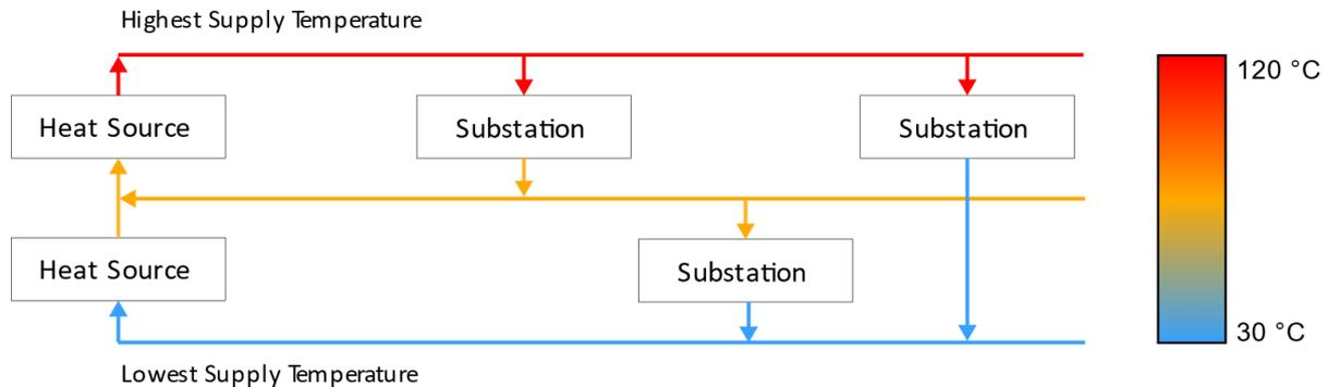
**Figure 5. Illustrative layout for the Warm – Multi-Level configuration, redrawn from [9]**
