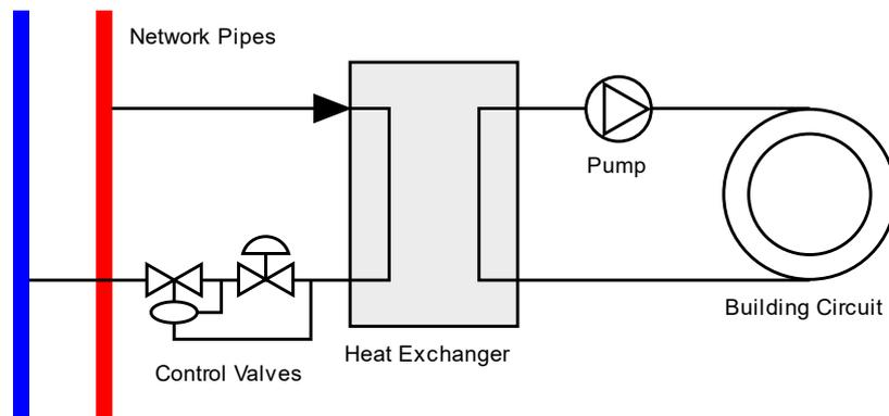
**Figure 4. Basic substation layout for indirect passive heating using a heat exchanger, based on [9]. Directions are reversed on the primary side for passive cooling**
