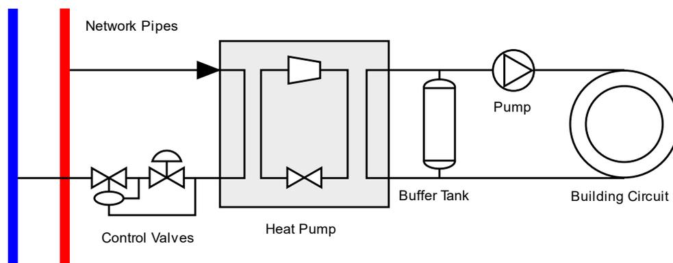
**Figure 8. Basic substation layout for active heating using a water-source heat pump and buffer tank**
