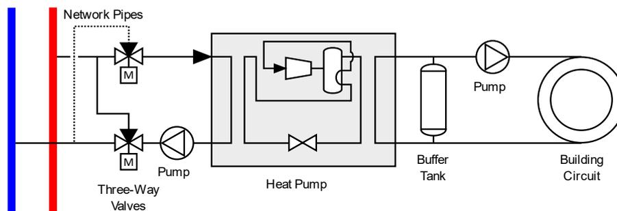
**Figure 12. Basic substation layout for active heating and cooling using a reversible water-source heat pump with four-way valve, buffer tank and bi-directional network exchange via three way valve arrangement**
