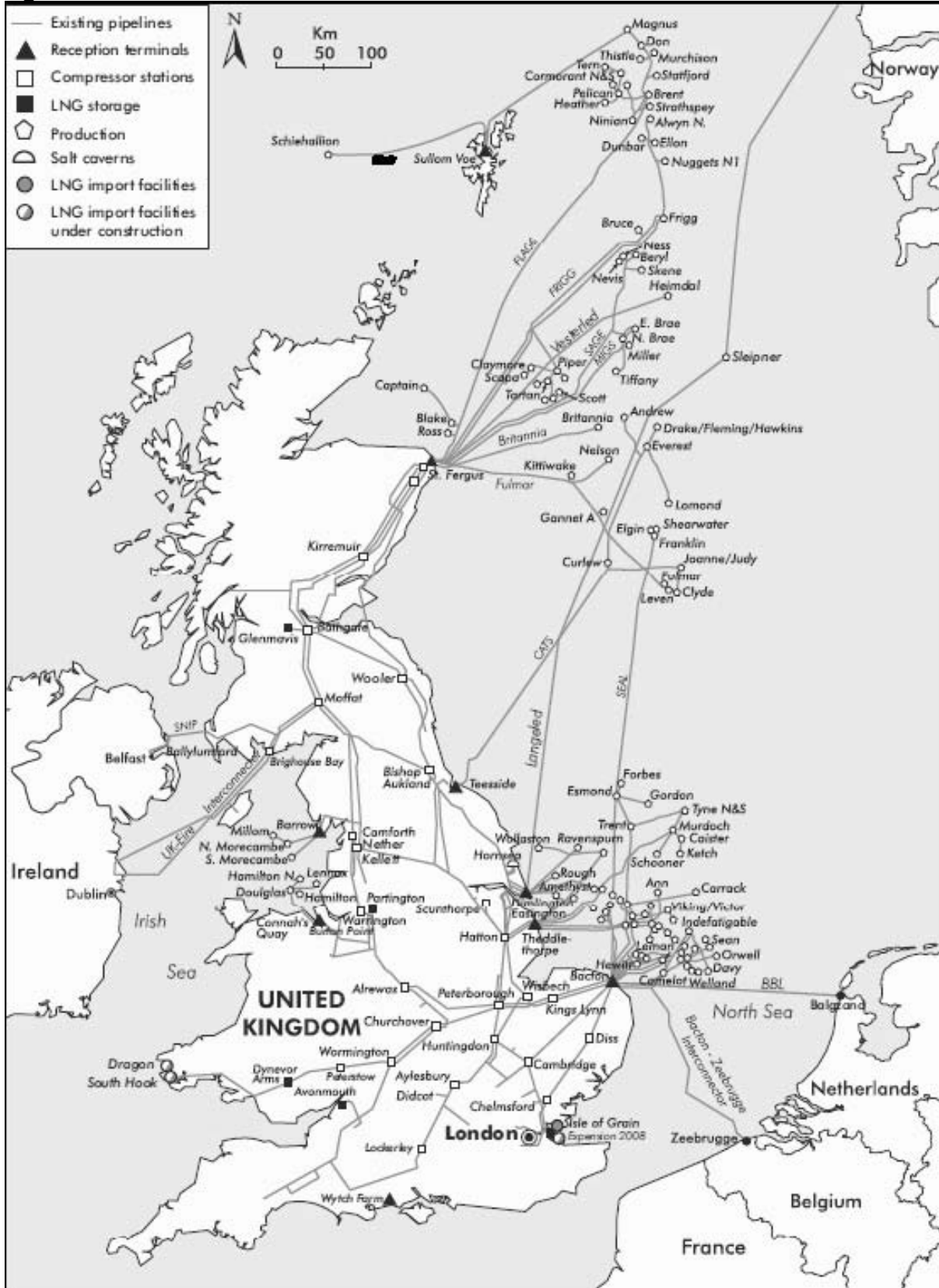
Figure 7: UK Gas Network
